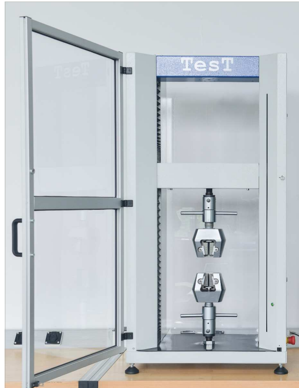
Universal Testing Machine 112.50kN with wedge grips for tensile testing
