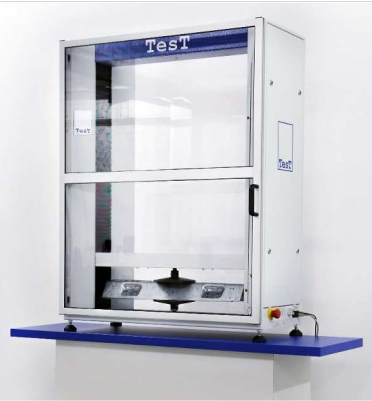
Testing machines for fixing elements For compressive, tensile and bendings tests
