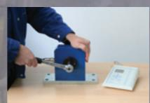
The combination of our sensors with the TesT measurement electronic and a special firmware allows straightforward determination of friction coefficients. Here, by measuring the parameters of force and
