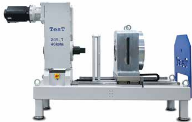
Friction coefficient test rig model 205.7 with 201.7
