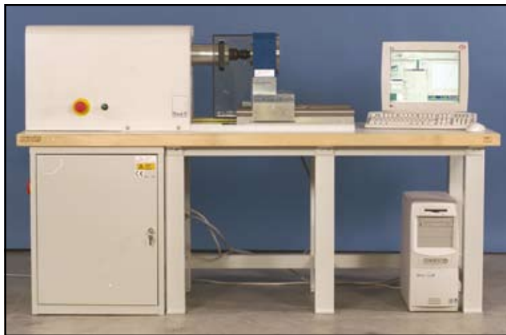
Test Screw-Testing-Machine from 35 Nm up to more than 15000 Nm Tests at different temperatures
