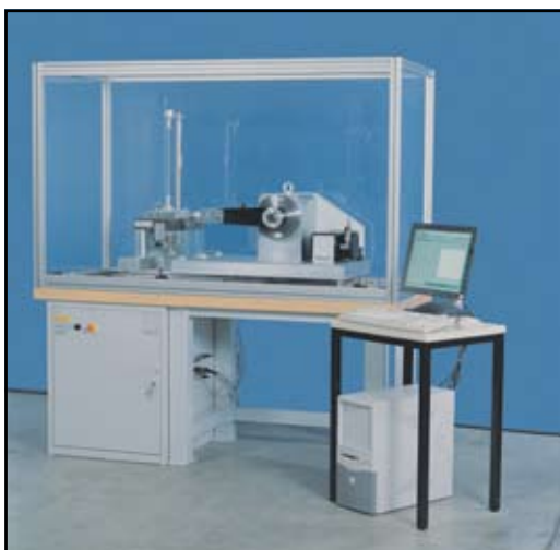
Test Vibration-Tester for screws between M6 and M16
