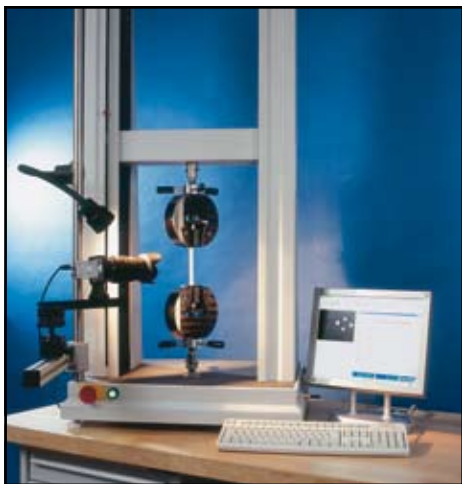
Test Universal-Testing-Machines optical extensometer
